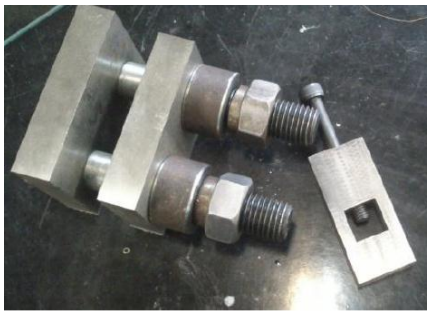
Figure 2. Fixture designed for shearing test
