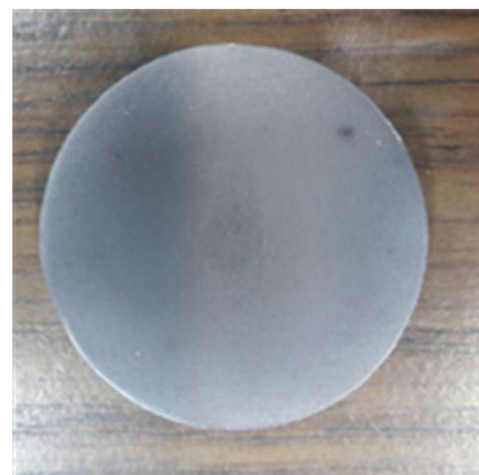
Figure 8. Picture of the Y3S specimen disc, 40 mm in diameter and 2 mm thick, consolidated by SPS
