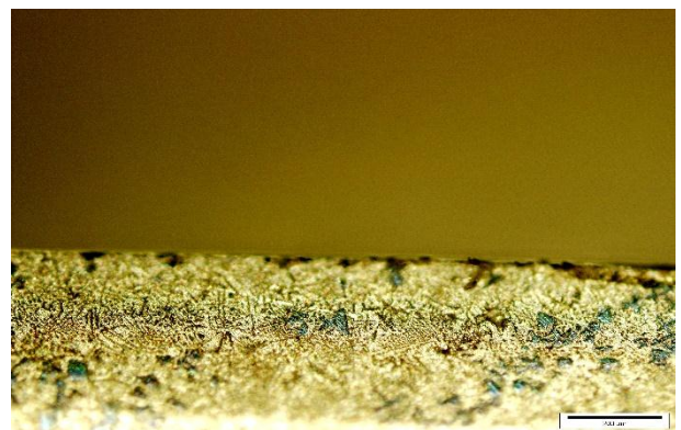
Figure 6. Distribution of reinforcing particles along the thickness from the outer wall to the inside (a to d) for the pouring temperature of 700 degrees Celsius and preheat 300 degrees ( Scale bar is 200 μm)
