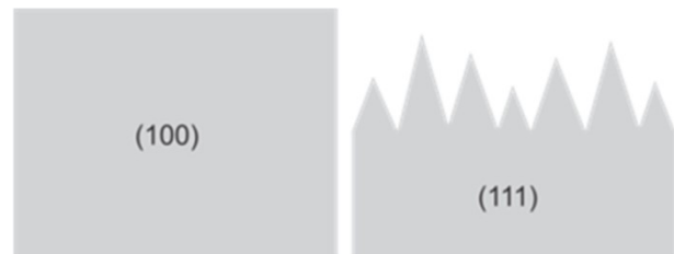
Figure 1. Schematic of silicon surface before and after etching
