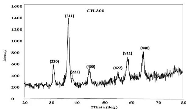
**Figure 1.** XRD pattern of pure  $\text{Co}_3\text{O}_4$  (CH) sample after calcination at 300 °C for 2 h
