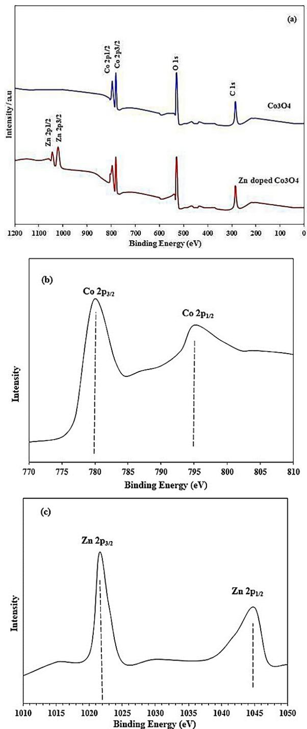
**Figure 4.** XPS spectra of the pure  $\text{Co}_3\text{O}_4$  and Zn doped  $\text{Co}_3\text{O}_4$  mesoporous nanoparticles, scanned in (a) Broad scan XPS analysis of Pure  $\text{Co}_3\text{O}_4$  and Zn doped  $\text{Co}_3\text{O}_4$  sample, high-resolution XPS spectra of (b) Co 2p, (c) Zn 2p, and (d) O 1s spectra for ZCH sample calcined at 300
