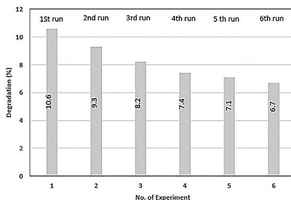
**Figure 6.** The reproducibility of the ZCH-300 catalyst for MB photodegradation for six cycles)
