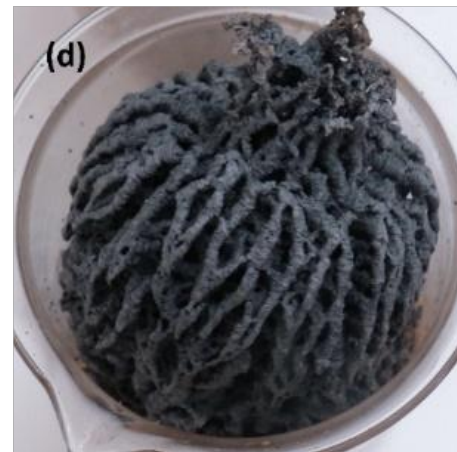
Figure 1. (a): Gelation, (b): initiation, (c); the auto-combustion process, and (d): the burnt and porous product of Y-type precursor synthesized via sol-gel auto-combustion method.
