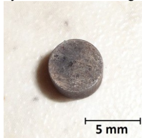
Figure 9. Image of nanostructured pin after wear test.
