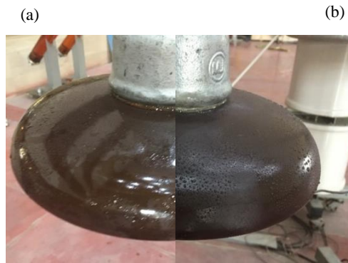
Figure 5. Leakage currents test for (a) Uncoated and (b) coated insulators.
