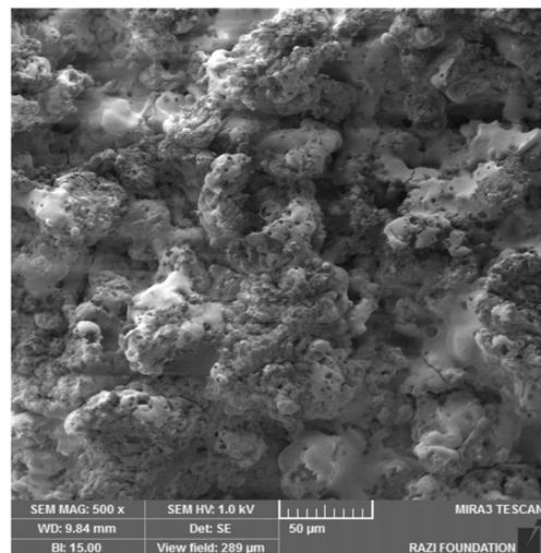
Figure 4. FESEM image of deposited feedstocks on the titanium substrate via plasma spray process
