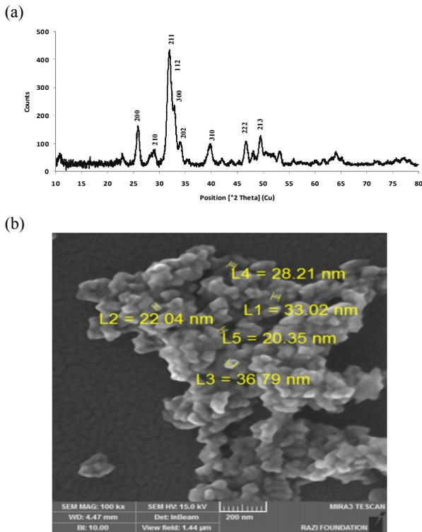
Figure 1. (a) XRD pattern and (b) FESEM image of synthesized hydroxyapatite
