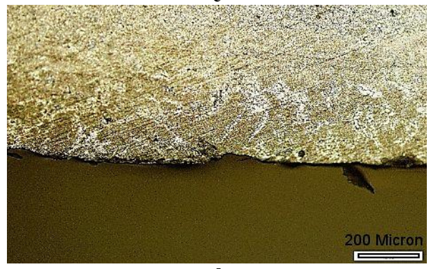
Figure 6. Distribution of reinforcing particles along the thickness from the outer wall to the inside (a to d) for the pouring temperature of 700 °C and preheat 300 °C
