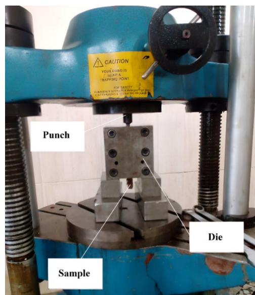
Figure 3. The extruding operation in the SSE process
