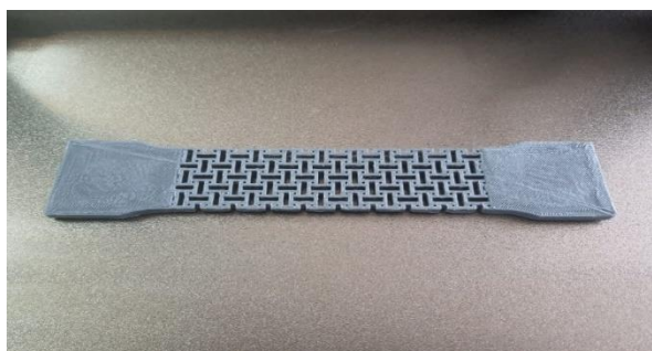
Figure 4. Complex-shaped SiC/polymer green part fabricated by FFF using the selected printing parameters, demonstrating the capability of the developed processing conditions for producing geometrically complex structures.
