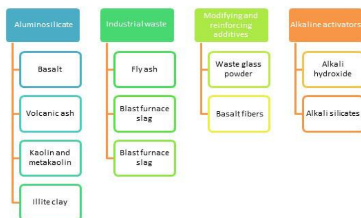
Figure 1. Classification of raw materials suitable for the production of geopolymer-based ceramics.
