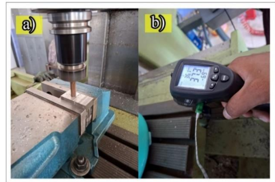
Figure 1. (a) Performing the Milling Process and (b) Real-Time Temperature Monitoring
