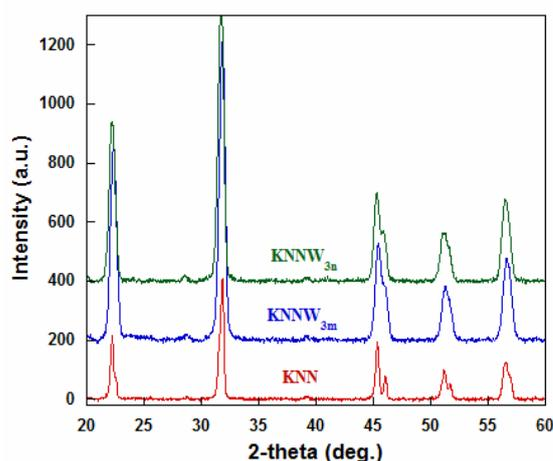
**Figure 1.** XRD patterns of KNN, KNNW<sub>3m</sub> and KNNW<sub>3n</sub> powders after calcinations at 950°C.
