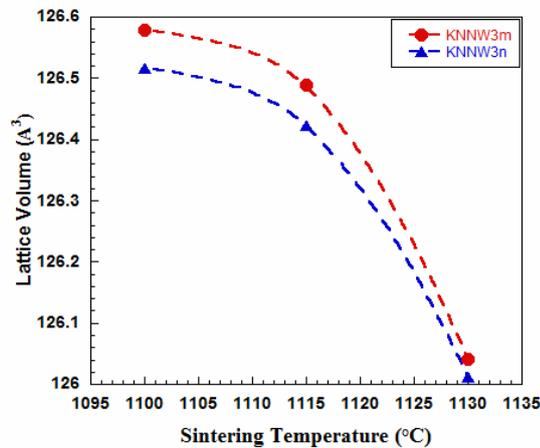
**Figure 5.** Variations in lattice volume with sintering temperature for  $\text{KNNW}_{3m}$  and  $\text{KNNW}_{3n}$  ceramics.
