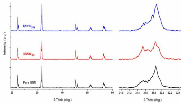
**Figure 3.** XRD patterns of KNN ceramics sintered at 1115°C.
