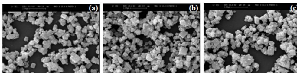
**Figure 2.** SEM micrographs of the powders (a) KNN, (b) KNNW<sub>3m</sub>, (c) KNNW<sub>3n</sub> calcined at 950°C for 4h.
