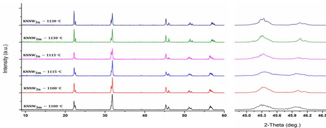
**Figure 4.** XRD patterns of  $\text{KNNW}_{3m}$  and  $\text{KNNW}_{3n}$  ceramics sintered at 1100-1130°C.
