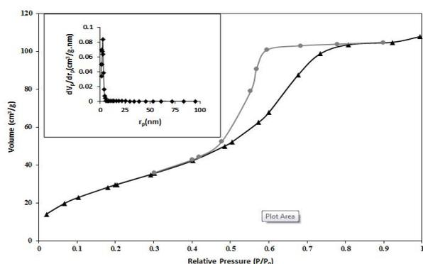
**Figure 5.** Nitrogen adsorption (▲) and desorption (●) isotherms for TiO<sub>2</sub> NPs in presence of NSAC. The inset shows BJH plot of this product.
