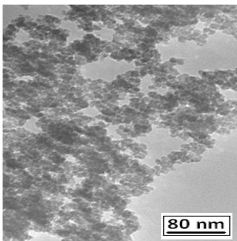
**Figure 2.** TEM image of titania NPs synthesized in presence of NSAC
