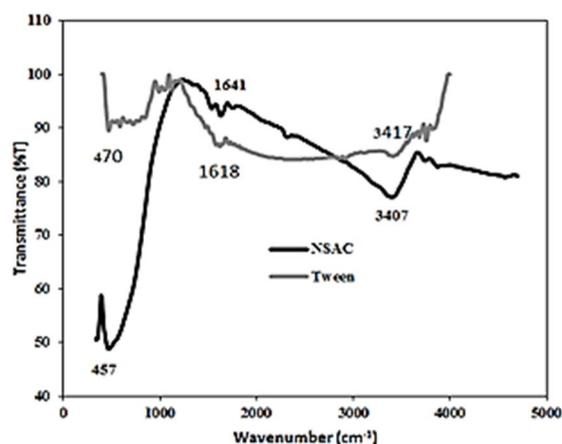
**Figure 4.** FTIR spectra for TiO<sub>2</sub>nanospheres synthesized by adding NSAC and Tween 40.
