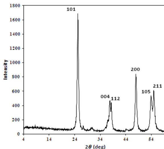
**Figure 6.** XRD pattern of TiO<sub>2</sub> nanoparticles prepared in presence of NSAC.
