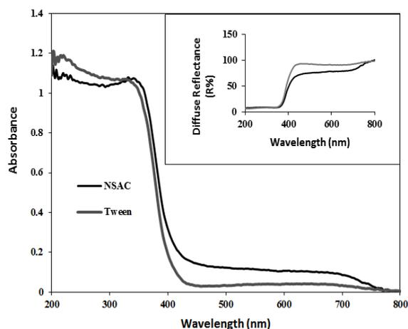
**Figure 3.** UV-absorbance spectra for TiO<sub>2</sub>nanospheres synthesized by adding NSAC and Tween 40.
