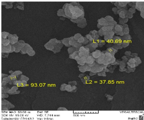
**Figure 2.** SEM micrograph of the synthesized titanium dioxide.
