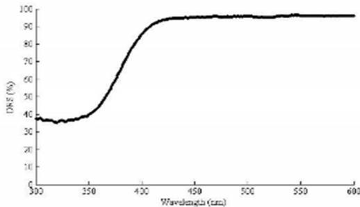
**Figure 4.** Diffuse reflectance spectra (DRS) versus wavelength for the synthesized titanium dioxide
