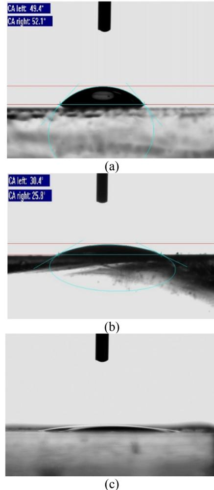
**Figure 5.** Contact angle measurement: a) in the dark room, b) under UV-ray for 20 min, c) under UV-ray for 40 min
