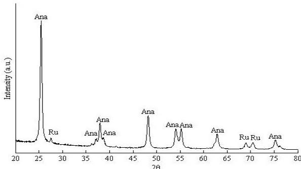
**Figure 1.** XRD pattern of the synthesized titanium dioxide
