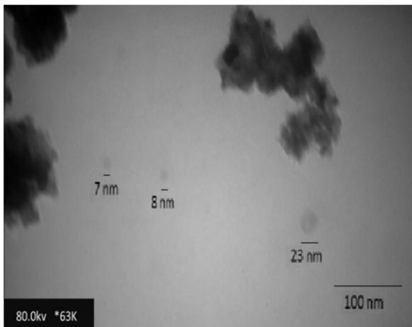
**Figure 3.** TEM image of the synthesized titanium dioxide
