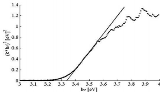
**Figure 5.**  $(K*hv)^2$  versus  $hv$  plot of the synthesized  $TiO_2$
