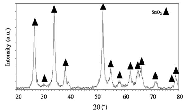
**Figure 2.** The XRD pattern of SCNSm sintered at 1200°C for 1h, revealing only the tetragonal structure of SnO<sub>2</sub>
