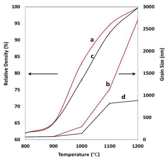
**Figure 4.** The plots of variations in relative density and grain size of undoped SnO<sub>2</sub> with temperature (a and c), and the corresponding plots for the sample doped with 0.05mol% Sm<sub>2</sub>O<sub>3</sub> (b and d)
