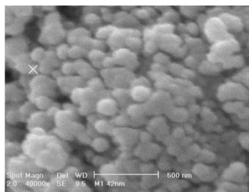
**Figure 1.** The SEM micrograph of the sample SCNSm doped with 0.05mol% Sm<sub>2</sub>O<sub>3</sub> calcined at 700°C for 2h
