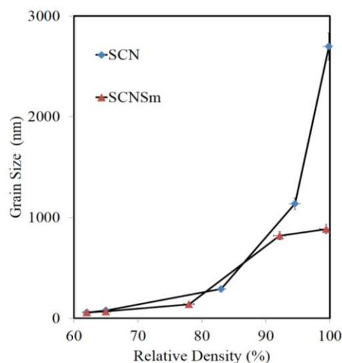
**Figure 5.** The mean grain size as a function of the relative density for undoped SnO<sub>2</sub> sample and the one doped with 0.05mol% Sm<sub>2</sub>O<sub>3</sub>, sintered at 800°C, 900°C, 1000°C, 1100°C, and 1200°C for 1h
