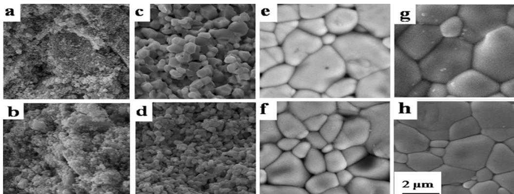
**Figure 3.** The SEM micrographs of the samples without and doped with 0.05mol%  $\text{Sm}_2\text{O}_3$  sintered at temperatures of  $900^\circ\text{C}$  (a,b),  $1000^\circ\text{C}$  (c,d),  $1100^\circ\text{C}$  (e,f), and  $1200^\circ\text{C}$  (g,h) for 1h
