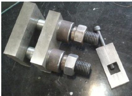
Figure 2. Fixture designed for shearing test
