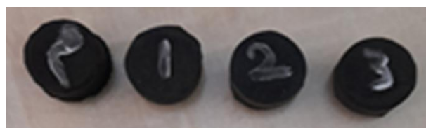
Figure 6. Examples of baked mixtures for a hardness test
