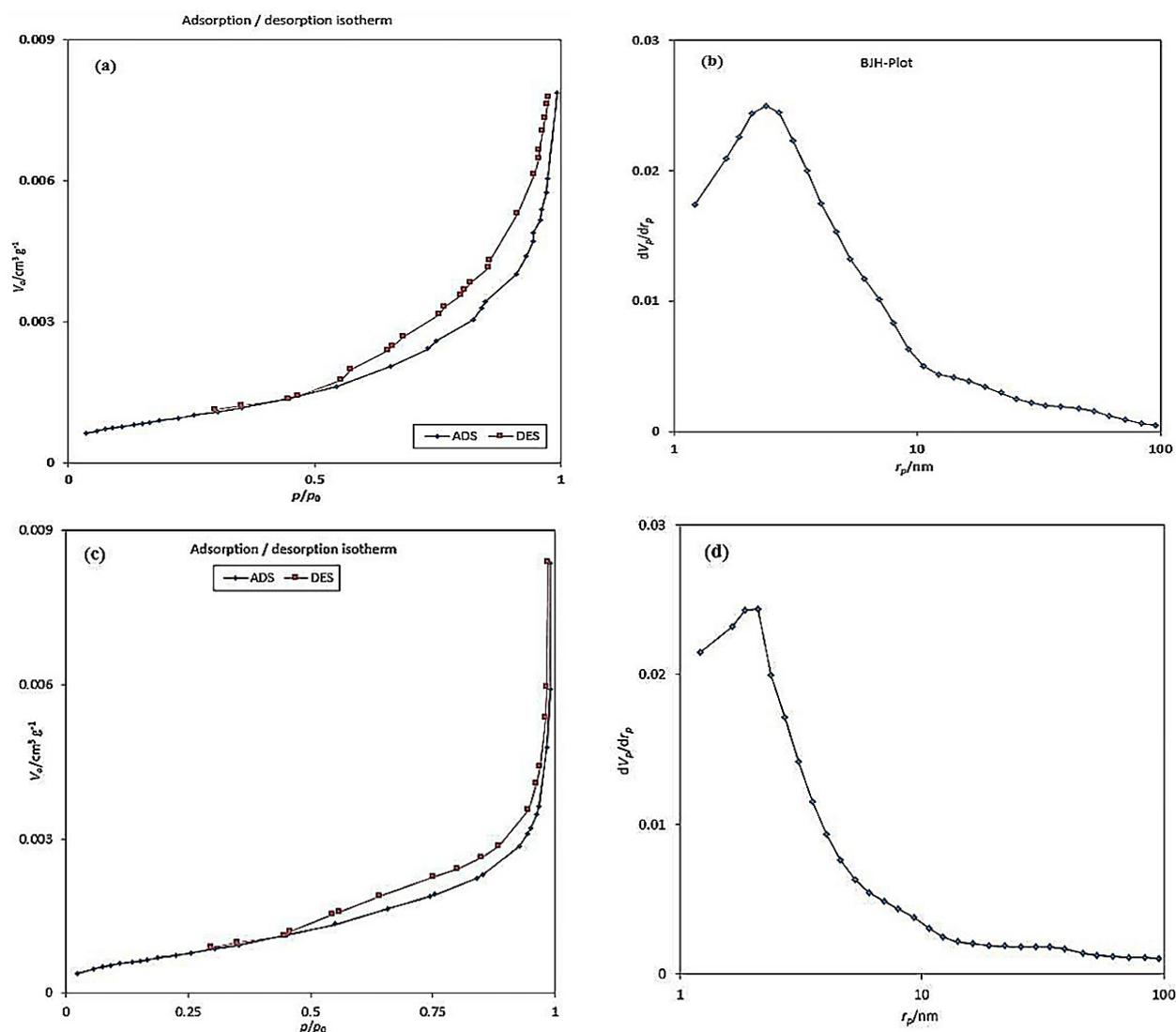
**Figure 3.** N<sub>2</sub> physisorption isotherms (BET) and pore size distribution (BJH) of CH (a,b) and ZCH (c,d) hydrothermally mesoporous nanoparticles calcined at 300 °C
