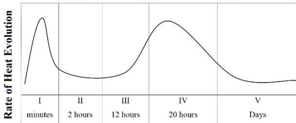
**Figure 6.** The heat of cement hydration vs. time
